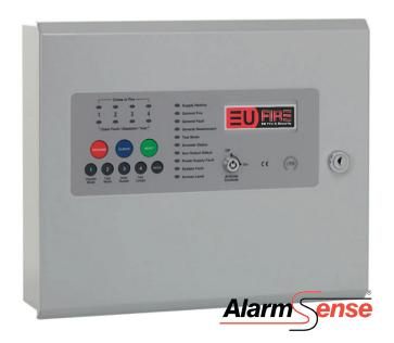
The AlarmSense PLUS is a 4 - 12 zone Apollo Fire Detectors AlarmSense protocol two-wire conventional control panel with integral power supply & space for standby batteries.
